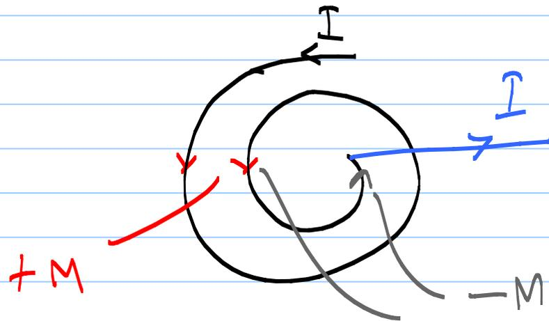
$\Rightarrow$  build inductors with large inner diameters
