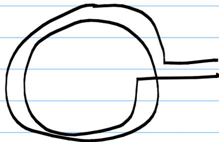
nH inductors require several 100s of  $\mu\text{m}$  to mm of length
