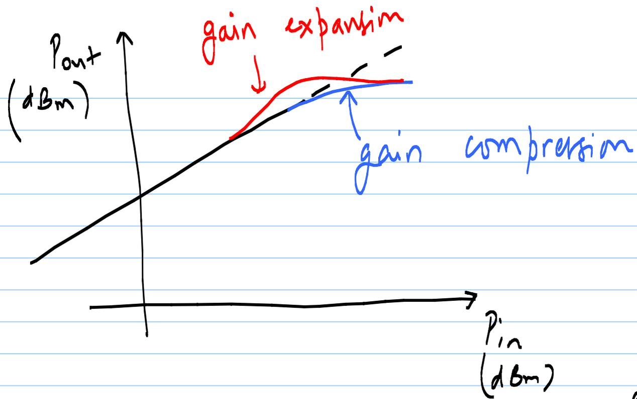
fundamental term:  $\alpha_1 + \frac{3\alpha_3 A^2}{4}$  — gain compression at large  $V_{GS} - V_T$
