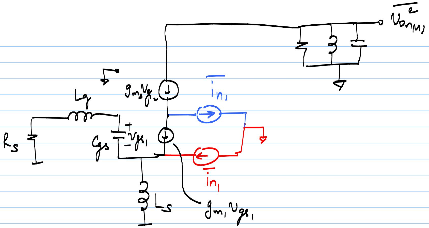
$$\begin{aligned} \overline{v_{onM_1}} &= \left[ \frac{R_d}{1 + R_d g_m} \right]^2 \cdot \overline{i_{n_1}}^2 \quad \cancel{\text{?}} \\ &= \left[ \overline{i_{n_1}} \times (g_m R_s + 1) \cdot R_d - \overline{i_{n_1}} \cdot R_d \right]^2 ?? \end{aligned}$$
