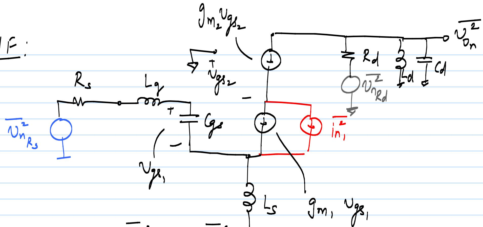
$$F = 1 + \frac{\bar{V}_{o_n}^2 M_1}{\bar{V}_{o_n}^2 R_s} + \frac{\bar{V}_{o_n}^2}{\bar{V}_{o_n}^2 R_1}$$
