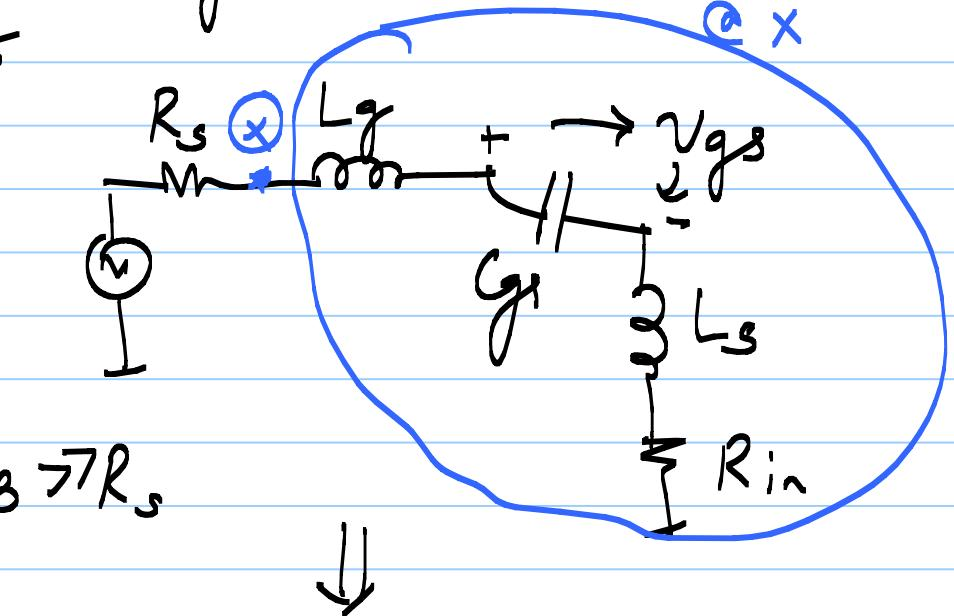
$$Q_{in} = \frac{1}{2R_s(\omega(g_s))} = \frac{\omega(L_s + L_g)}{2R_s}$$
