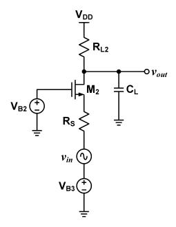
Given:  $V_{DD}=1.3V$ ,  $R_S=50\Omega$ ,  $R_{L2}=0.8k\Omega$  and  $C_L=1pF$ . The operating points of  $M_2$  are as follows:  $I_d=1mA$ ,  $V_{ds}=0.9V$ ,  $g_m=8mA/V$ ,  $g_{ds}=0.3mA/V$ ,  $g_{mb}=2.1mA/V$ ,  $C_{gs}=30fF$ ,  $C_{gd}=13fF$ ,  $C_{gb}=0.8fF$ ,  $C_{db}=26fF$ ,  $C_{sb}=29fF$ . Bulk of  $M_2$  is grounded.
