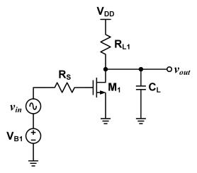
Given:  $V_{DD}=1.3V$ ,  $R_S=50\Omega$ ,  $R_{L1}=0.9k\Omega$  and  $C_L=1pF$ . The operating points of  $M_1$  are as follows:  $I_d=1mA$ ,  $g_m=8.2mA/V$ ,  $g_{ds}=0.3mA/V$ ,  $g_{mb}=2.2mA/V$ ,  $C_{gs}=31fF$ ,  $C_{gd}=14fF$ ,  $C_{gb}=1fF$ ,  $C_{db}=28fF$ ,  $C_{sb}=31fF$ . Bulk of  $M_1$  is grounded.
