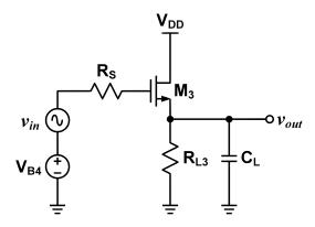
Given:  $V_{DD}=1.3V$ ,  $R_S=50\Omega$ ,  $R_{L3}=0.5k\Omega$  and  $C_L=1pF$ . The operating points of  $M_3$  are as follows:  $I_d=1mA$ ,  $g_m=7.4mA/V$ ,  $g_{ds}=0.3mA/V$ ,  $g_{mb}=1.8mA/V$ ,  $C_{gs}=25fF$ ,  $C_{gd}=11fF$ ,  $C_{gb}=0.4fF$ ,  $C_{db}=21fF$ ,  $C_{sb}=23fF$ . Bulk of  $M_3$  is grounded.
