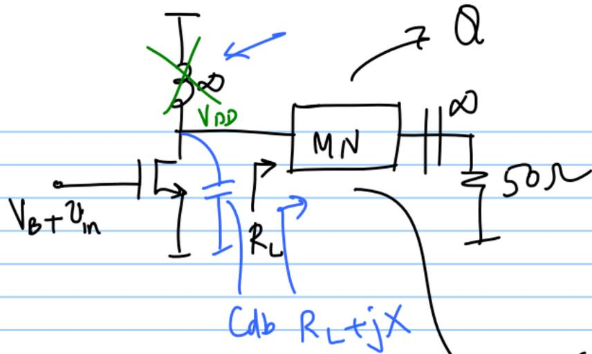
e.g.  $R_L = 12.5 \Omega$ ,  $P_{out_{max}} = 160 \text{ mW}$
