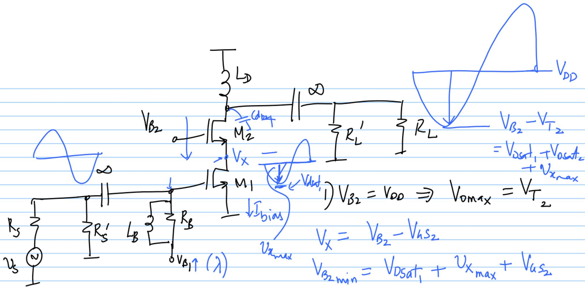
So far: Linear / Class A PAs  $\theta_c = 360^\circ$  "conduction angle"
