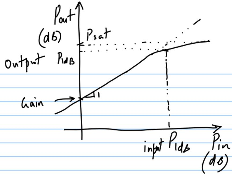
e.g.  $V_{\text{DD}} = 1.8\text{V} \Rightarrow P_{\text{sat}} = 8.1\text{mW}$
