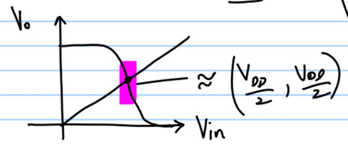
max amplitude  $\approx V_T$  (linear operation)
