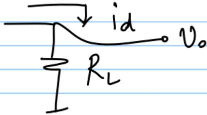
$i_d = \frac{V_o}{R_L}$  → set to triode limit
