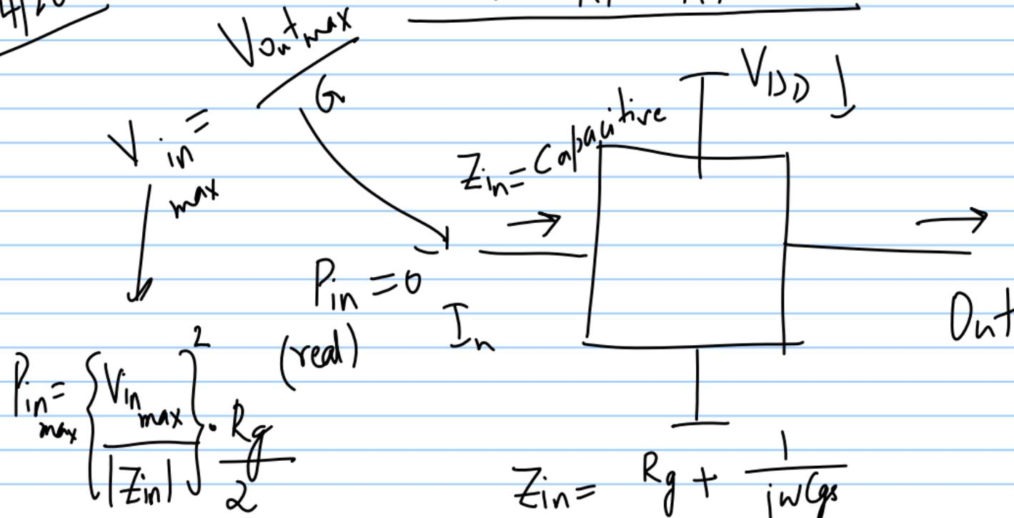
$$P_{in\_max} = \frac{\left\{ \frac{V_{in\_max}}{|Z_{in}|} \right\}^2 \cdot R_g}{2}$$
