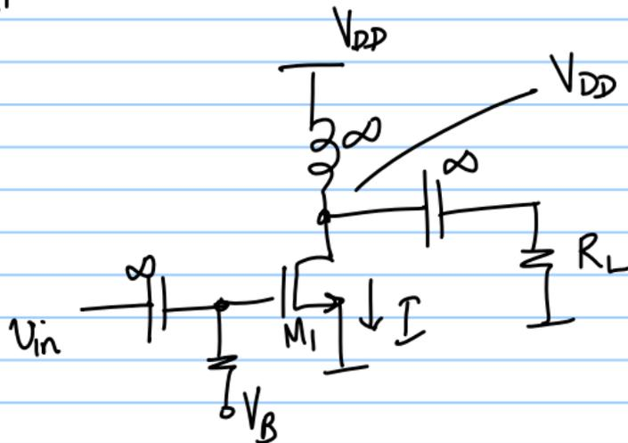
$$V_{O_{DC}} = V_{DD}$$
