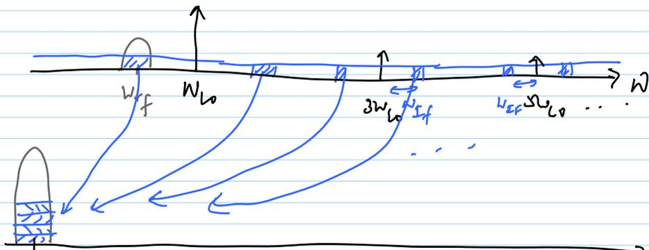
$$\frac{N_{\text{out}}}{\Delta f} = \frac{4kT\sigma^2}{g_m} \times \left(\frac{2}{\pi} g_m R_L\right)^2 \times \left(1 + \frac{1}{3^2} + \frac{1}{5^2} + \dots\right) \times 2$$
