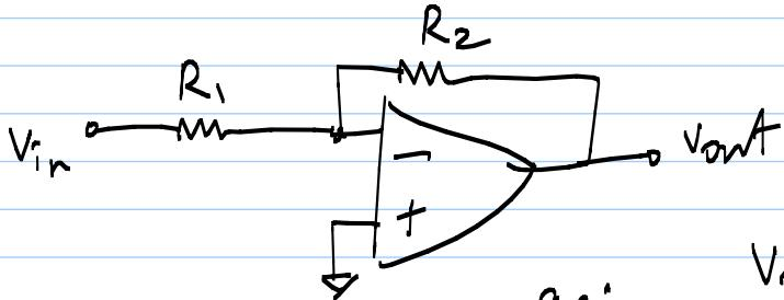
$$\text{gain } \frac{V_{out}}{V_{in}} = -\frac{R_2}{R_1}$$
