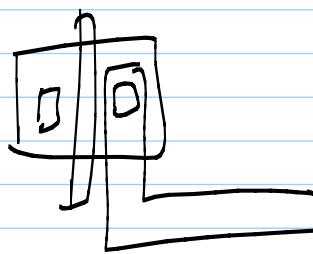
metal lines can affect parasitic cap to device nodes!
