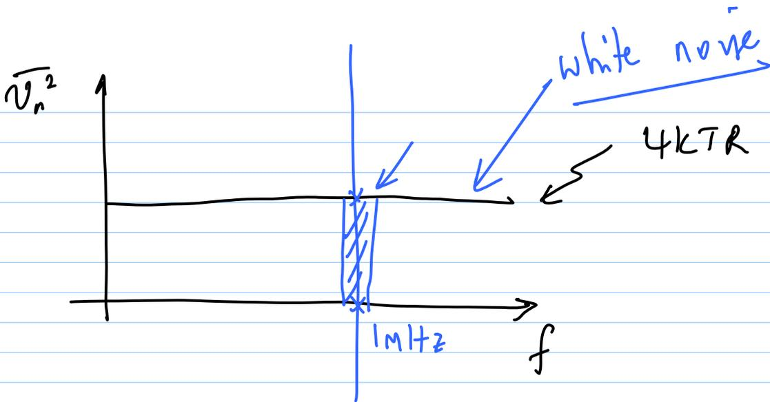
$$\overline{v_n^2} \Big|_{1MHz} = 4kTR \left( \frac{V^2}{Hz} \right) \times 1(Hz)$$
