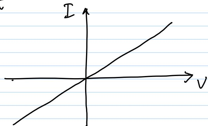
\* passive 1-part :  $V \cdot I \geq 0 \Rightarrow 1^{\text{st}} \& 3^{\text{rd}}$  quadrants
