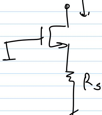
V<sub>CVS</sub> — Common drain amp.
