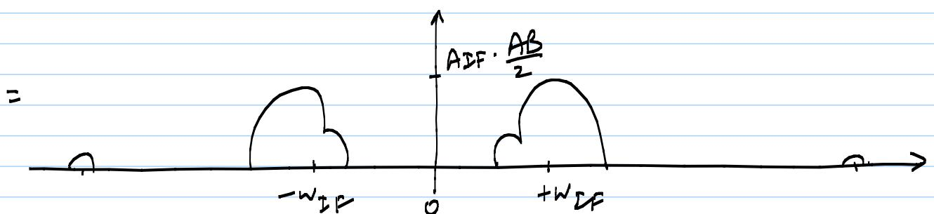
\* For easy IF design (ie. high gain, high Q filtering etc.), we want small  $\omega_{IF}$
