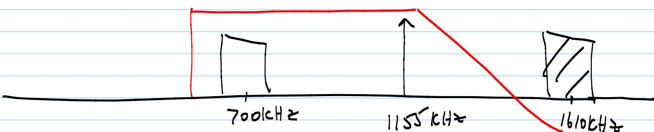
\* Images are out-of-band for channels  $\geq 710\text{kHz}$
