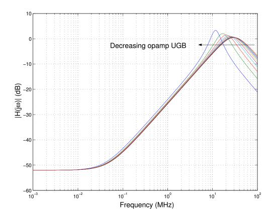
Figure 5.3: Variation of stop band response in a biquad with varying opamp UGB The criteria for compensation is that
