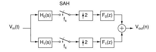
Figure 3.5: Setup to measure SFDR in a 2-channel HFB based ADC
