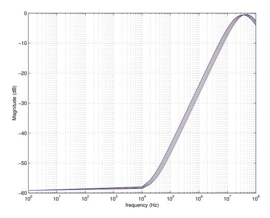
Figure 5.13: Tunable frequency response. Simulated  $f_c$  ranges from 33 to 48 MHz
