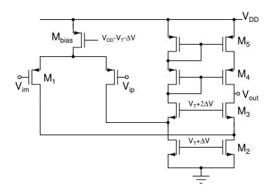
Figure 4.9: pMOS folded cascode gain boosting amplifier
