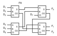
Figure 4.24: Thermometer to binary converter for 3-bit Flash ADC
