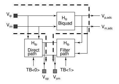
Figure 5.14: Setup for measuring frequency response of the biquad
