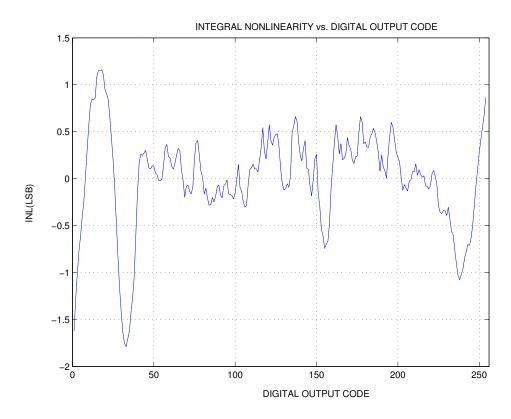
Figure 6.9: INL plot for full scale input at 40 MHz sampling rate
