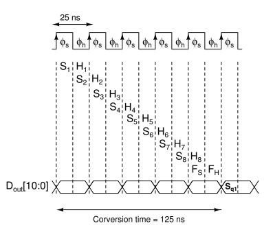
Figure 4.25: Signal flow in the DEC block
