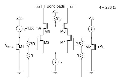
Figure 5.15: Test buffer schematic
