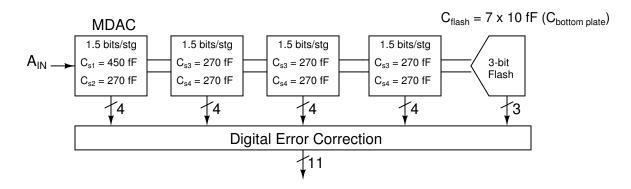
Figure 4.2: Architecture of the 10-bit pipelined ADC
