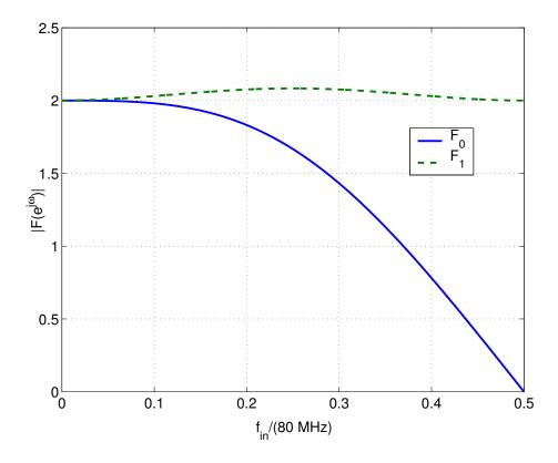
Figure 3.7: 2 channel HFB synthesis filters for 32-tap filters
