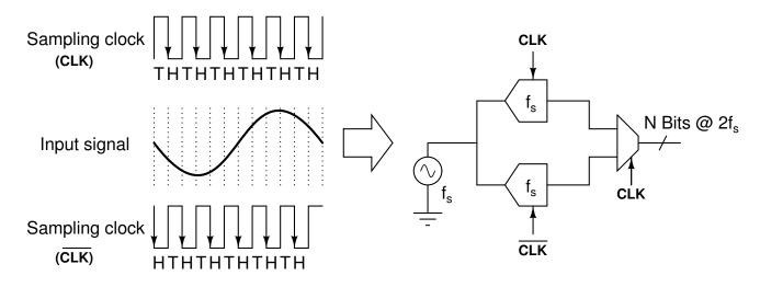
Figure 3.1: 2-channel time interleaved ADC
