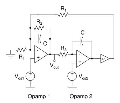
Figure 7.10: Effect of input referred opamp offsets
