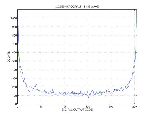
Figure 6.5: Output histogram for full scale input at 40 MHz sampling rate
