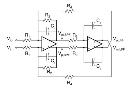
Figure 5.1: Biquad schematic
