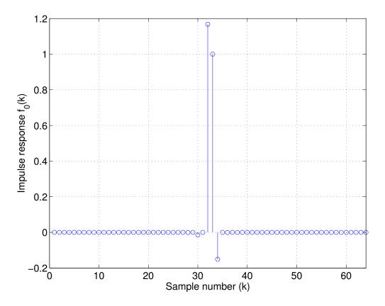
Figure 6.14: 64 tap impulse response of  $F_0(z)$
