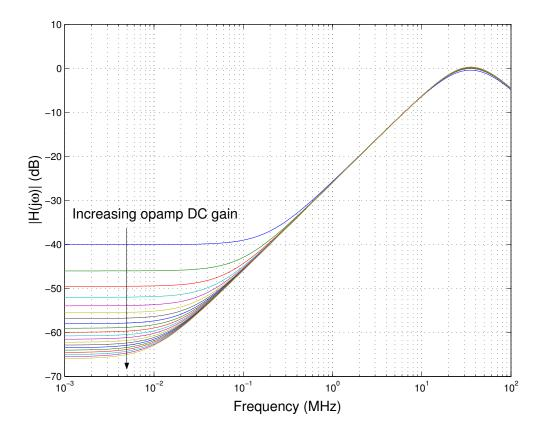
Figure 5.2: Variation of stop band response in a biquad with varying opamp DC gain
