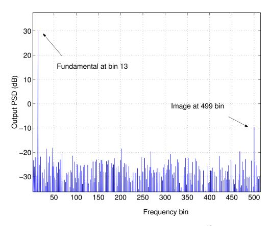
Figure 6.16: Output spectrum to input of  $f_{in} = \frac{13}{512} f_s$
