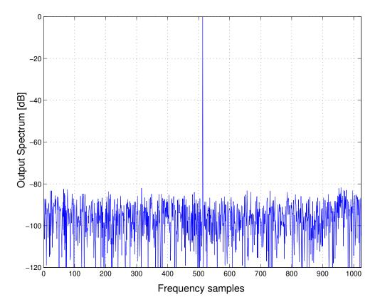
Figure 4.33: ADC output spectrum for a 10 MHz input
