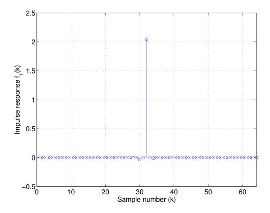
Figure 6.15: 64 tap impulse response of  $F_1(z)$
