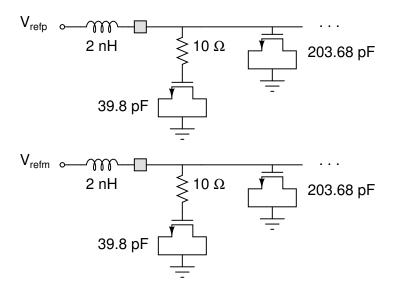
Figure 4.30: Bypass capacitor on external voltage references
