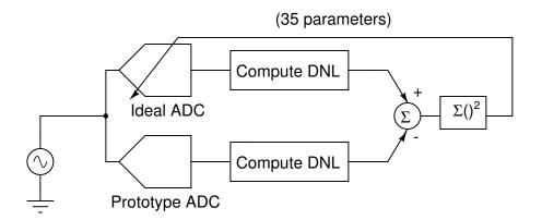
Figure 7.3: Estimation technique to fit prototype behavior to ideal ADC with programmable parameters using histogram test
