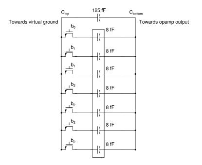
Figure 5.12: Capacitor tuning
