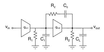
Figure 5.5: Small signal equivalent showing pole-zero compensation
