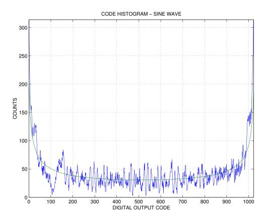
Figure 7.5: Measured Histogram at 10-bit level
