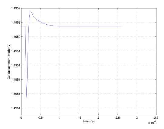
Figure 5.7: Common mode feedback loop stability
