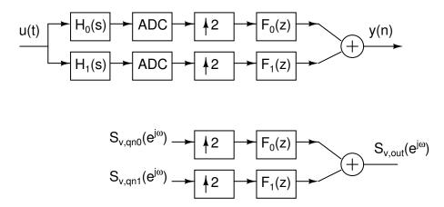
Figure 3.9: Computing SNR at the output in a 2-channel HFB based ADC
