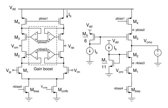
Figure 4.12: Biasing - Generation of pbias2, nbias3
