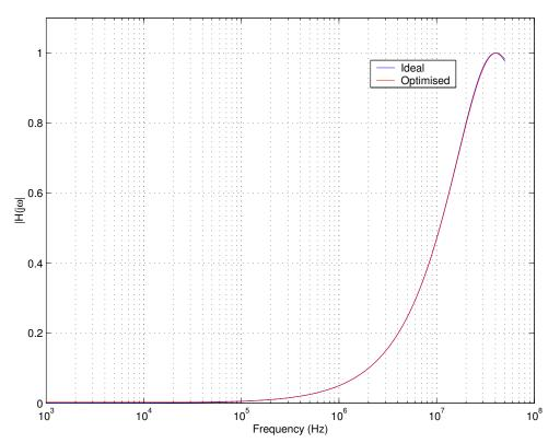
Figure 5.10: Ideal, Obtained responses after [R<sub>1</sub>,R<sub>2</sub>,R<sub>3</sub>,C] optimization
