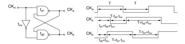
Figure 4.29: Non-overlapping clock generator
