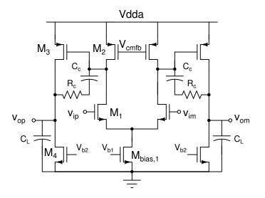
Figure 5.4: Opamp topology used in the biquad realization
