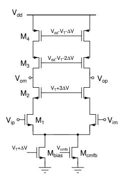
Figure 4.7: Telescopic opamp without the gain boosting amplifiers
