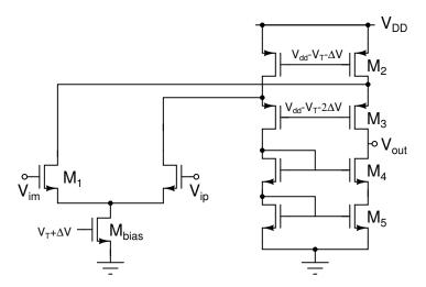
Figure 4.8: nMOS folded cascode gain boosting amplifier
