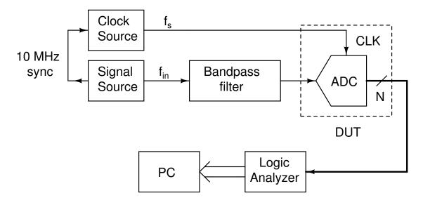
Figure 2.2: Setup for characterizing an ADC
