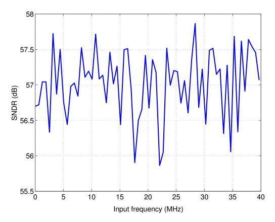
Figure 3.12: SNR simulation for a 2-channel HFB realized using "All pass & Biquad" analog filters
