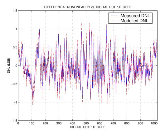
Figure 7.8: Measured and Estimated DNL at 10-bit level
