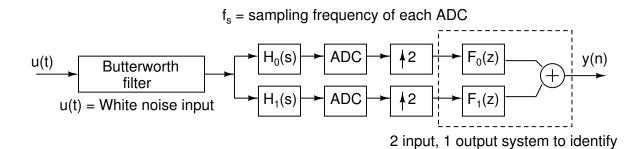
Figure 3.8: Synthesis filter identification using LMSE criteria
