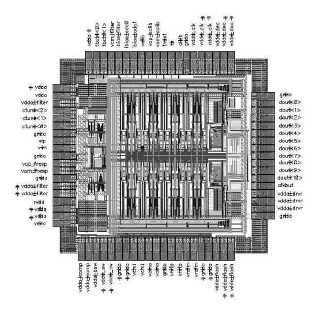
Figure 5.21: 2-channel HFB ADC layout.
