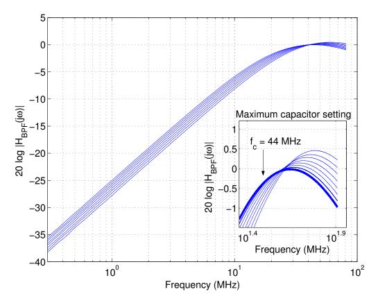
Figure 6.11: Frequency response of the bandpass filter for 7 capacitor settings
