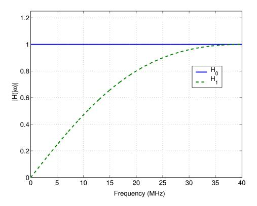
Figure 3.6: 2 channel HFB analysis filters
