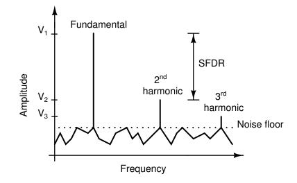
Figure 2.1: Spectrum of the output of an ADC to a single-tone input
