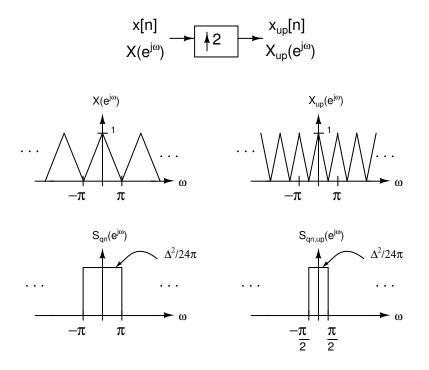
Figure 3.10: Interpolation by factor 2
