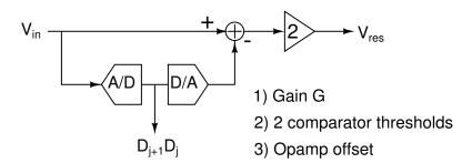
Figure 7.1: 3 MDAC stage parameters that affect the stage characteristic
