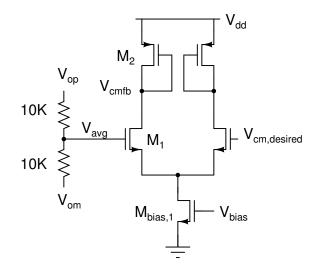
Figure 5.6: Common mode feedback loop
