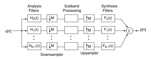
Figure 3.2: M-channel discrete-time filter bank
