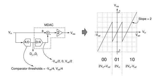
Figure 4.4: MDAC stage input-output characteristic
