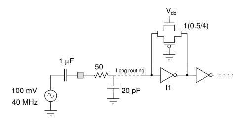
Figure 4.28: Converting sine wave clock to square wave
