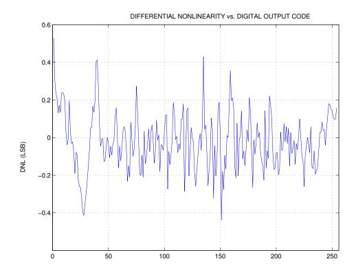
Figure 6.7: DNL plot for full scale input at 40 MHz sampling rate
