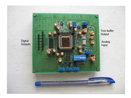
Figure 6.2: PCB designed for prototype characterization
