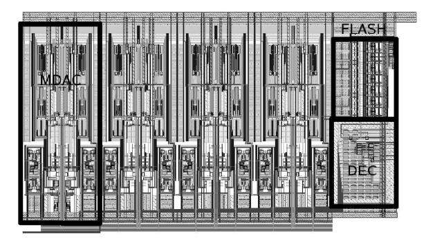
Figure 4.32: Layout of the sub band ADC
