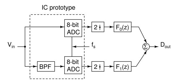
Figure 6.13: Equivalent model at 8-bit accuracy level
