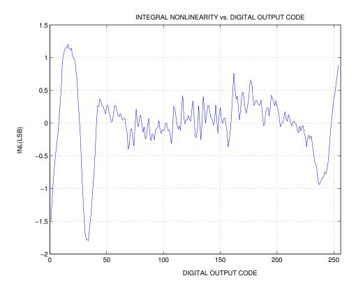
Figure 6.8: INL plot for full scale input at 20 MHz sampling rate
