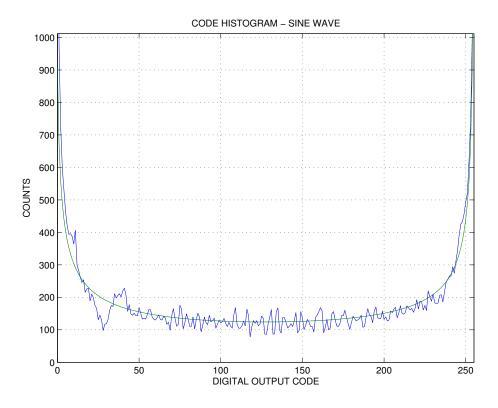
Figure 6.4: Output histogram for full scale input at 20 MHz sampling rate
