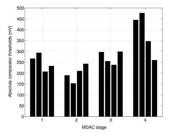
Figure 7.9: Absolute comparator thresholds in the 4 MDAC stages
