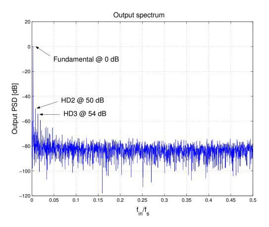
Figure 6.10: Output spectrum for Channel 0 ADC using 4K point FFT
