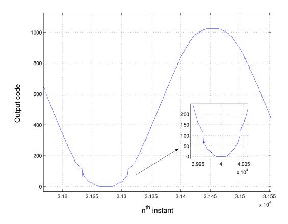
Figure 7.4: Distortion introduced in sine wave in negative cycle only indicative of errors in MDAC comparator thresholds
