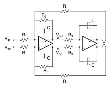
Figure 5.8: Biquad schematic
