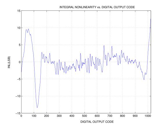
Figure 7.7: Measured INL at 10-bit level
