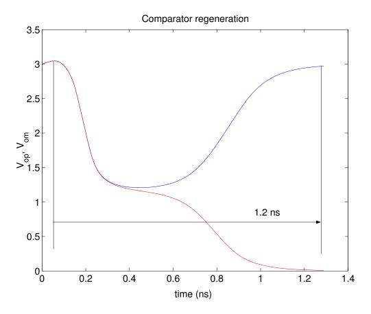
Figure 4.19: MDAC stage comparator regeneration
