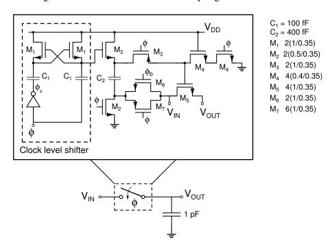
Figure 4.15: Schematic of bootstrapped switch
