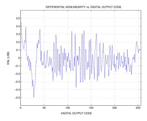
Figure 6.6: DNL plot for full scale input at 20 MHz sampling rate
