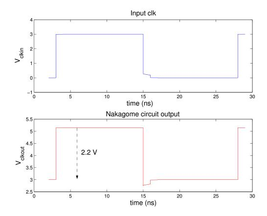
Figure 4.17: Nakagome charge pump output
