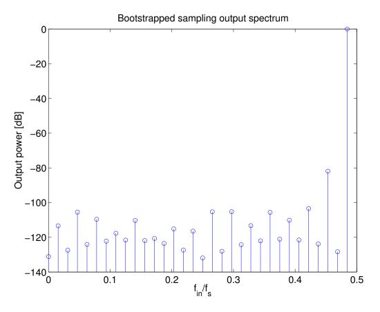
Figure 4.16: Output spectrum of the bootstrapped switch
