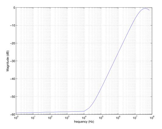
Figure 5.16: Frequency response. Simulated  $f_c = 10^{7.605} = 40.27 \text{ MHz}$
