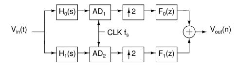
Figure 3.4: 2-channel HFB based ADC
