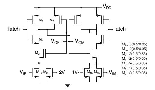
Figure 4.18: MDAC stage comparator
