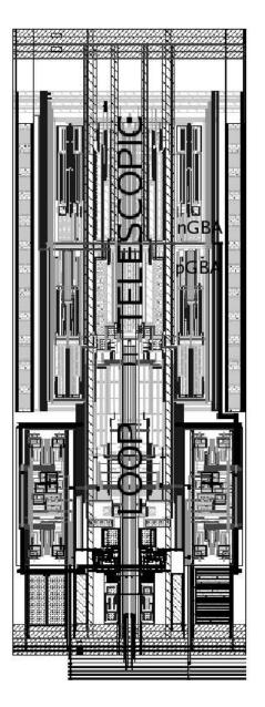
Figure 4.31: Layout of the MDAC stage
