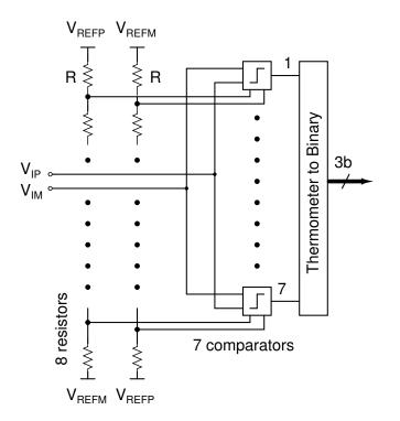
Figure 4.21: 3-bit Flash architecture
