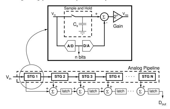
Figure 4.1: Architecture of a generic pipelined ADC
