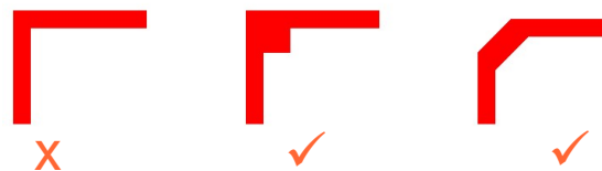
Bending of a high current line
