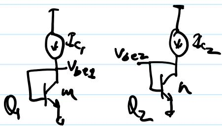
$$V_{be1} = V_T \ln\left(\frac{I_{c1}}{I_{S1}}\right) \quad \text{--- (1)}$$
