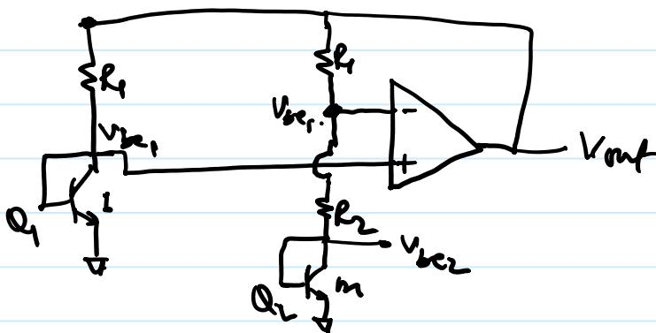
$$I_{R_2} = \frac{V_{be_1} - V_{be_2}}{R_2} = \frac{\Delta V_{be}}{R_2}$$
