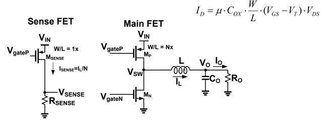
The width (W) of the Power MOSFET is X1000-10000 times the width of SENSEFET to reduce the power consumption.
