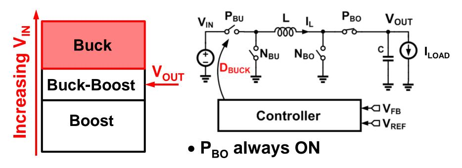
• D<sub>BUCK</sub> controls buck switches
