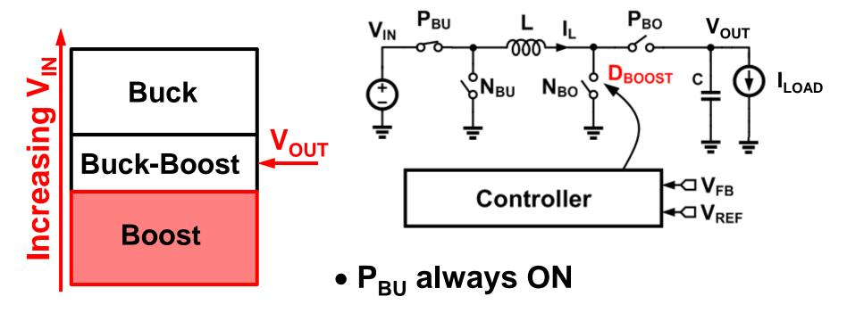
D<sub>BOOST</sub> controls boost switches
