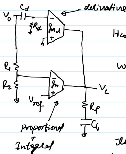
$$H_{\text{comp}}(s) = -\beta \frac{R_p g_m (1 + s/\omega_{z_1})(1 + s/\omega_{z_2})}{C_i s (1 + s/\omega_p)}$$
