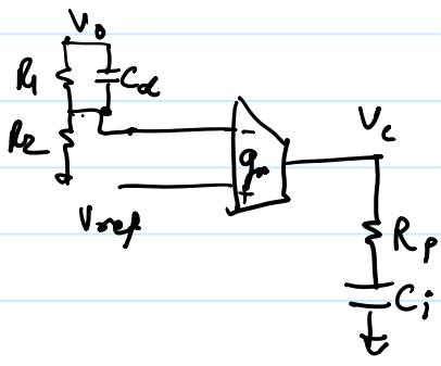
$$H_{\text{comp}}(s) = -\beta \frac{(1 + R_1 C_d s)}{(1 + \beta R_1 C_d s)} \left( g_m R_p + \frac{g_m}{C_i s} \right)$$
