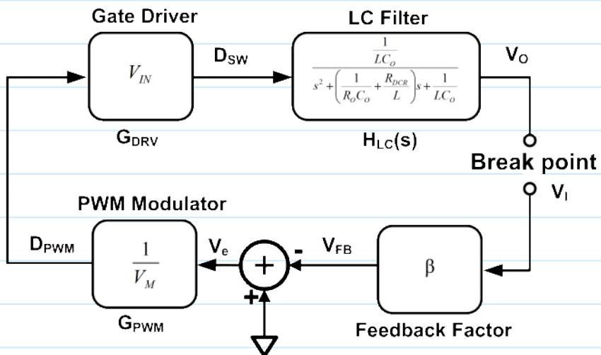
$$LG_u(s) = -\frac{R_2}{R_1 + R_2} \cdot \frac{V_{IN}}{V_M} \cdot \frac{1}{s^2 + \left( \frac{1}{R_o C_o} + \frac{R_{DCR}}{L} \right) s + \frac{1}{LC_o}}$$
