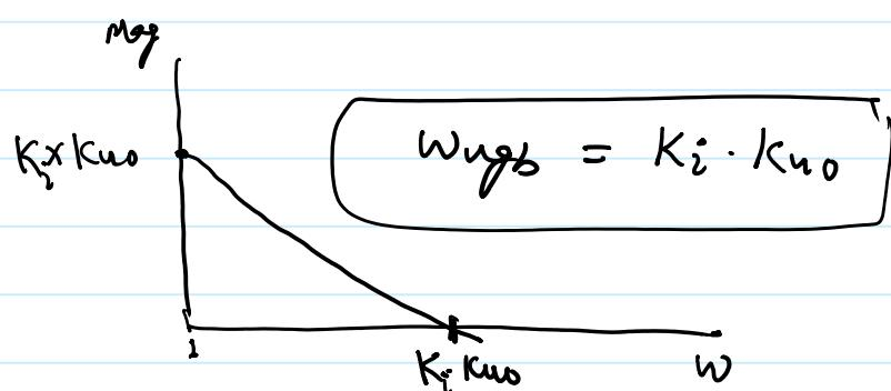
Provides an ideal compensation but not practical to realize as compensation zeroes can't be exactly placed at  $\omega_0$  due variation in parameters and component across varying operating conditions. Hence this type of compensation is not used.
