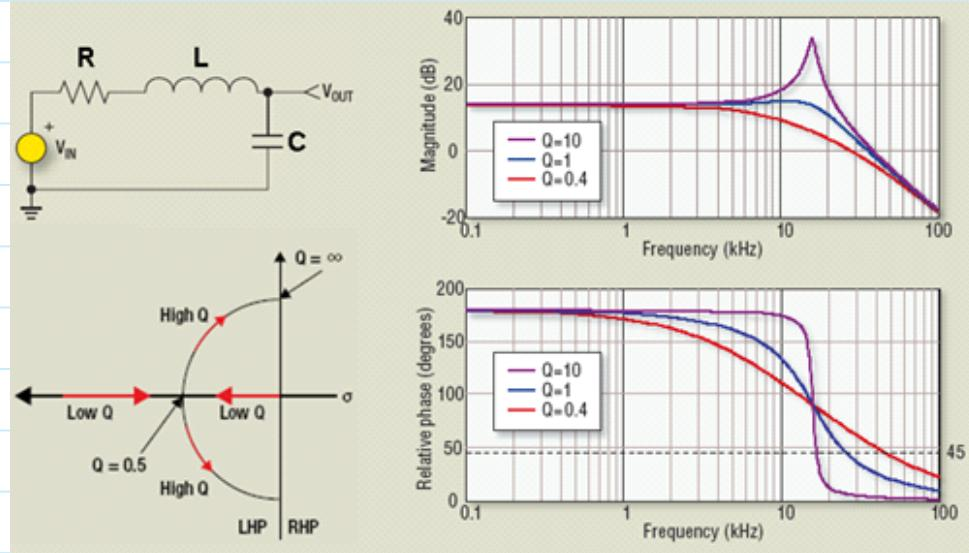
complex poles due to LC filter may cause  $90^\circ$ – $180^\circ$  phase shift around  $f_0$  (resonance freq.) and making system unstable.
