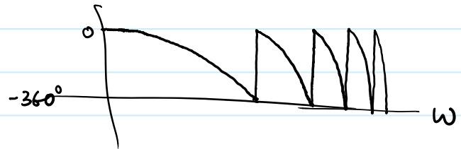
$$\theta = -2\pi + \omega = \frac{2\pi}{T_{sw}} = 2\pi f_{sw}$$
