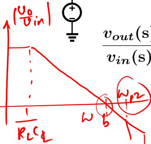
$$\frac{v_{out}(s)}{v_{in}(s)} = \frac{g'_m R_L}{1 + g'_m R_S} \frac{1}{\left(1 + \frac{C_S}{\left(g'_m + \frac{1}{R_S}\right)} s\right) (1 + R_L C_L s)}$$
