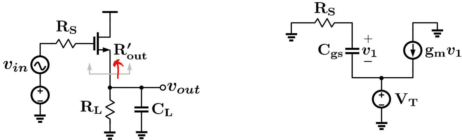
$$v_1 C_{gs} s + g_m v_1 = -I_T$$
