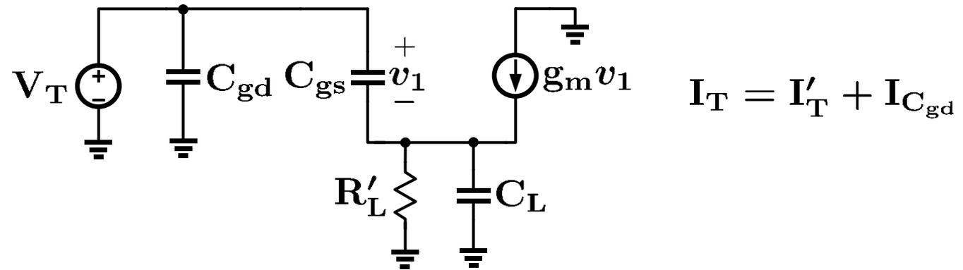
$$V_T = \frac{I'_T}{sC_{gs}} + (I'_T + \frac{g_m I_T}{C_{gs} s})(R'_L \parallel \frac{1}{C_L s})$$
