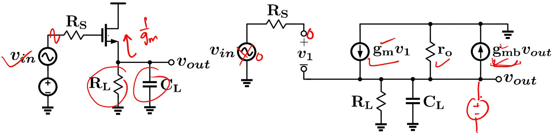
$$R'_L = r_o \parallel \frac{1}{g_{mb}} \parallel R_L$$
