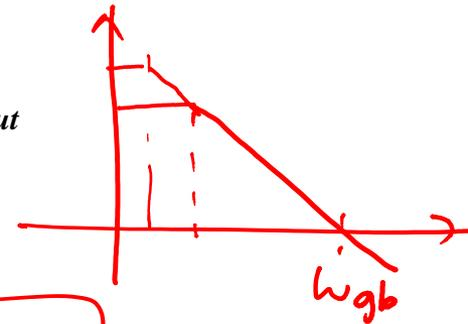
$$A_v(s) = -g_m R_{out} \frac{1 - sC_{gd}/g_m}{1 + s(C_{gd} + C_L)R_{out}}$$
