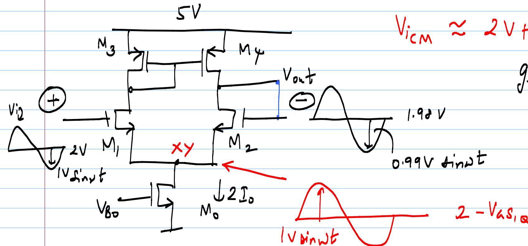
$$V_{iCM} \approx 2V_+ - 1V \sin \omega t$$
