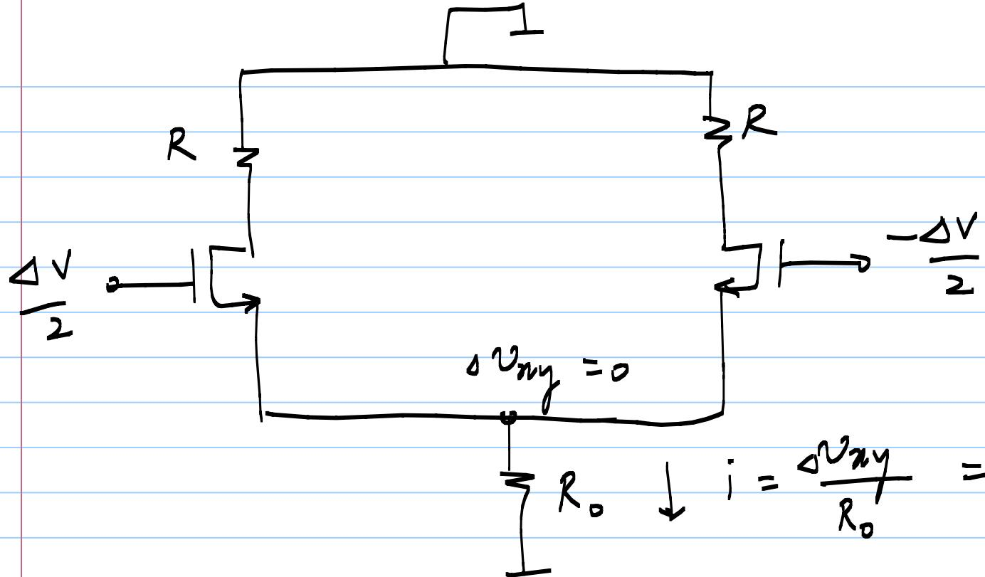
$i = \frac{\Delta V_{xy}}{R_0} = 0$  is the only possible state of the DM cir.
