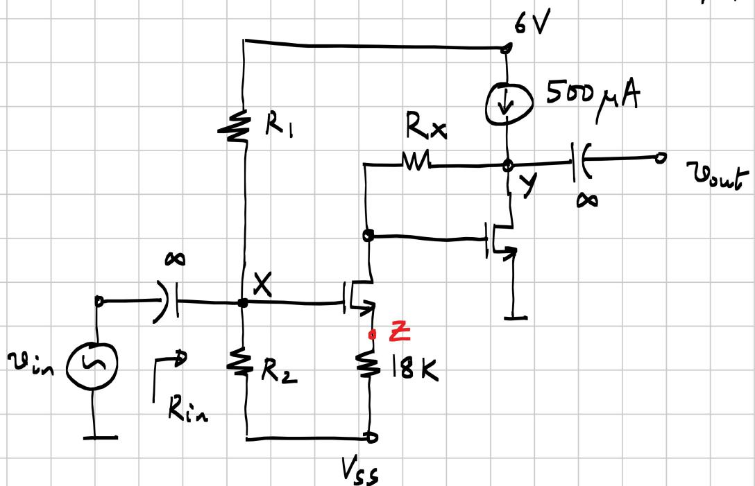
The quiescent currents through both transistors are equal. Determine  $R_x$ ,  $V_{ss}$ ,  $R_1$ , &  $R_2$  so that
