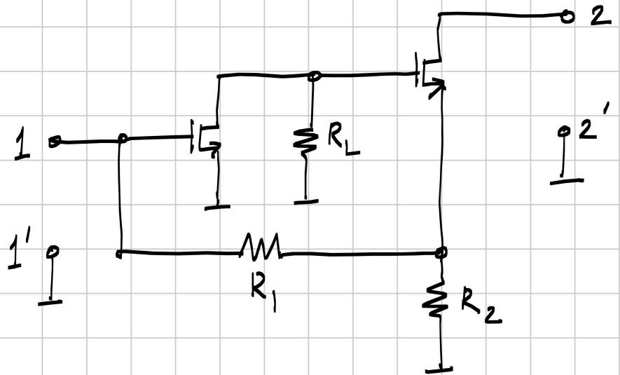
The circuit above is the incremental equivalent of an amplifier. The transistors have transconductances denoted by  $g_m$ .
