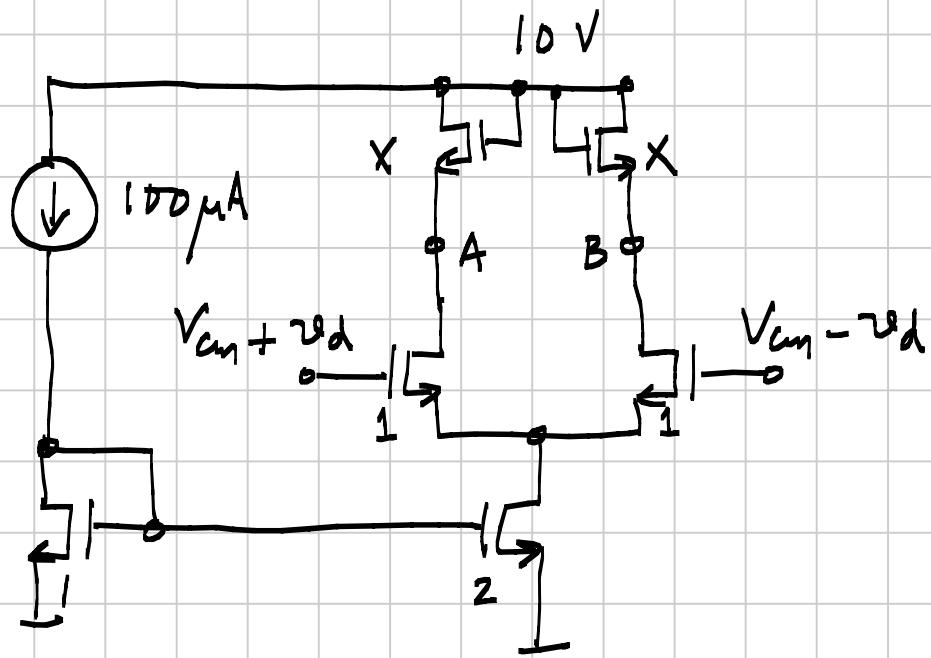
Determine the aspect ratio  $X$ , so that the incremental voltage between B & A is  $4V_d$ . What is the quiescent voltage at A?
