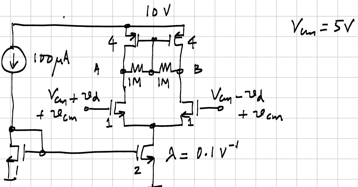
$\varphi_{cm}$  &  $\varphi_d$  are small signals. Only for the tail current source, use  $\lambda = 0.1 V^{-1}$ . Neglect  $\lambda$  to find the quiescent operating point.
