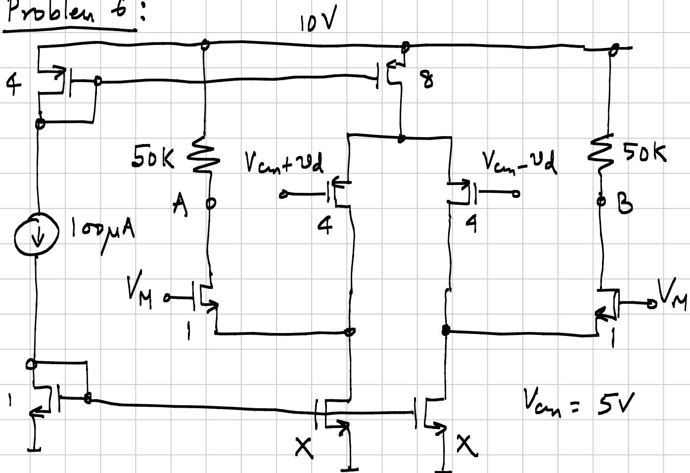
(a) Assuming all devices are in saturation, determine  $X$  so that the quiescent voltage at A & B is 5V.
