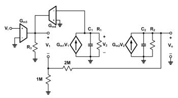
For the closed loop feedback system shown above  $G_{m1}$  = 25 mA/V,  $G_{m2}$  = 40 mA/V,  $G_{m3}$  = 1 mA/V,  $R_1$  = 1k $\Omega$ ,  $R_2$  = 100 $\Omega$ ,  $R_3$  = 1k $\Omega$ ,  $C_1$  = 100 pF,  $C_2$  = 1 nF,
