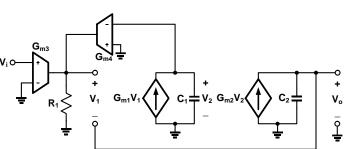
For the closed loop feedback system shown above  $G_{m1}$  = 4 mA/V,  $G_{m2}$  = 25mA/V,  $G_{m3}$  = 1 mA/V,  $R_1$  = 1k $\Omega,~C_1$  = 10 pF,  $C_2$  = 100 pF,
