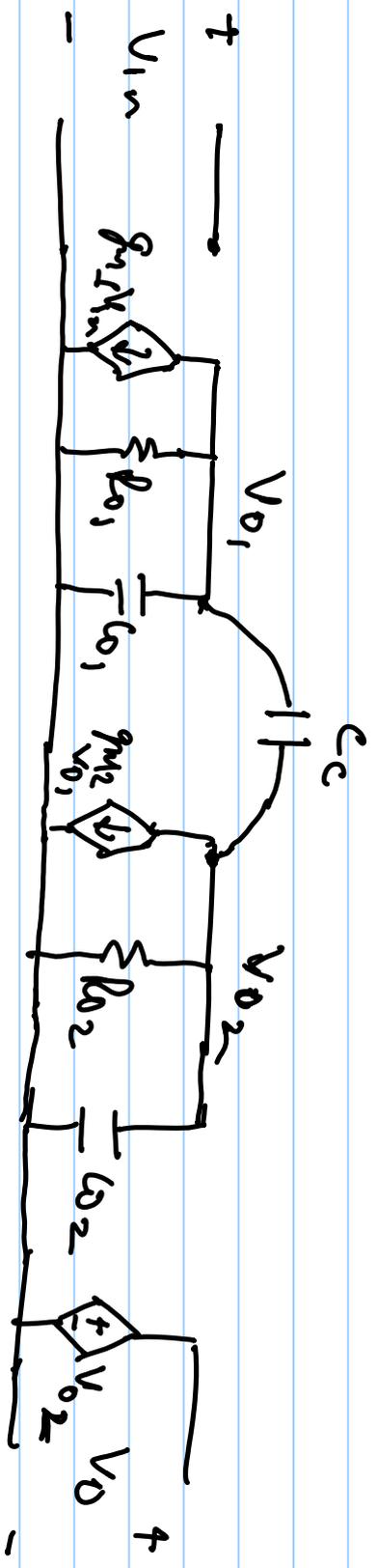
Apply KCL of  $V_{01}$   $G_{01} = \frac{1}{R_{01}}$  &  $G_{02} = \frac{1}{R_{02}}$
