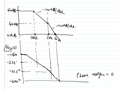
In order to increase the phase malgin or make the system stable, loop needs to be compensated.
