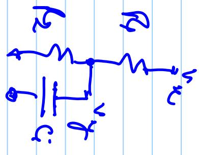
$$\frac{V_x(s)}{V_n(s)} = \beta = \frac{R_2}{R_1 + R_2} \cdot \alpha \frac{1}{\frac{1}{R_2 C s}} = \frac{R_2}{R_1 + R_2} \cdot \left(1 + \frac{1}{R_2 C s}\right)$$
