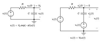
$$V_{o}(j\omega) = V_{i}(j\omega) \underbrace{\frac{1}{1+j\omega CR}}_{1+j\omega CR} + V_{x}(j\omega) \underbrace{\frac{j\omega CR}{1+j\omega CR}}_{1+j\omega CR}$$
