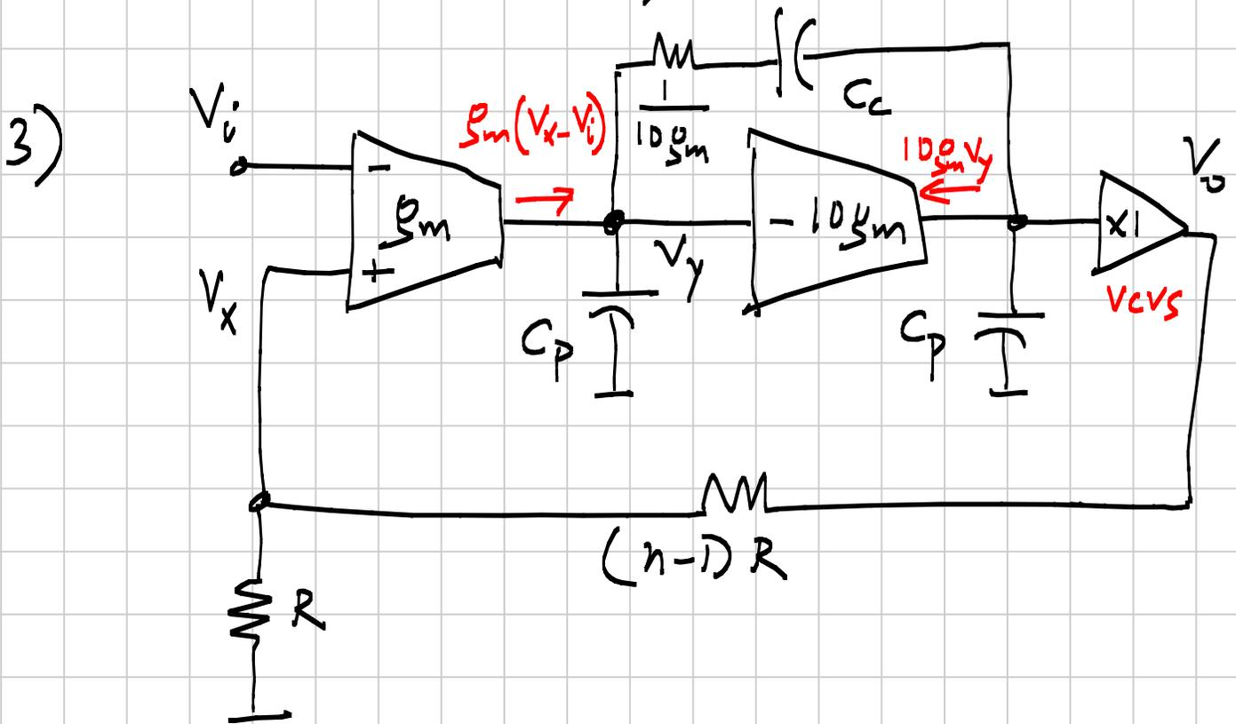
(a) Determine the closed loop DC gain.
