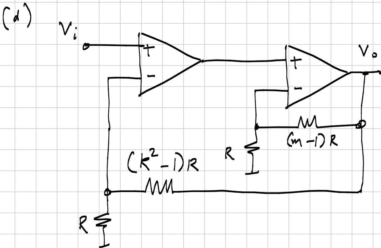
Determine the transfer functions of each of these amplifiers.
