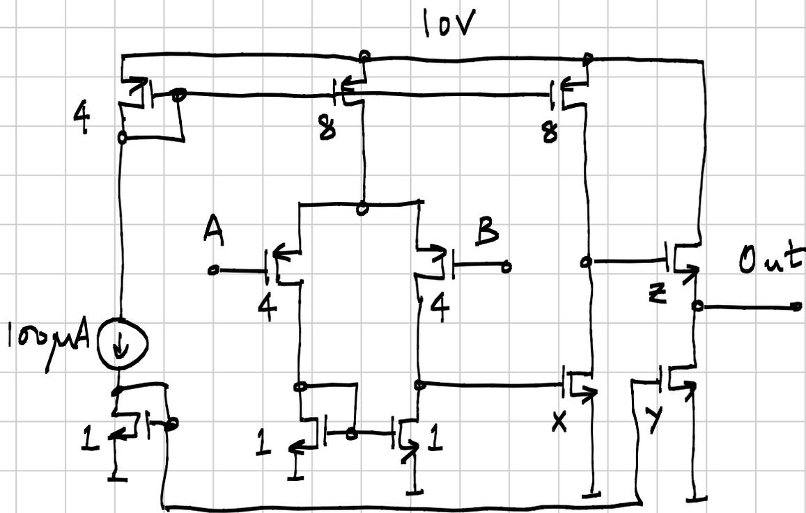
(c) The output of the opamp should be able to sink in 1 mA. Further, the output resistance should be  $500\ \Omega$ . Determine  $y$  &  $z$  for this to happen.
