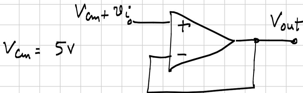
Determine the incremental gain and output impedance of the buffer.
