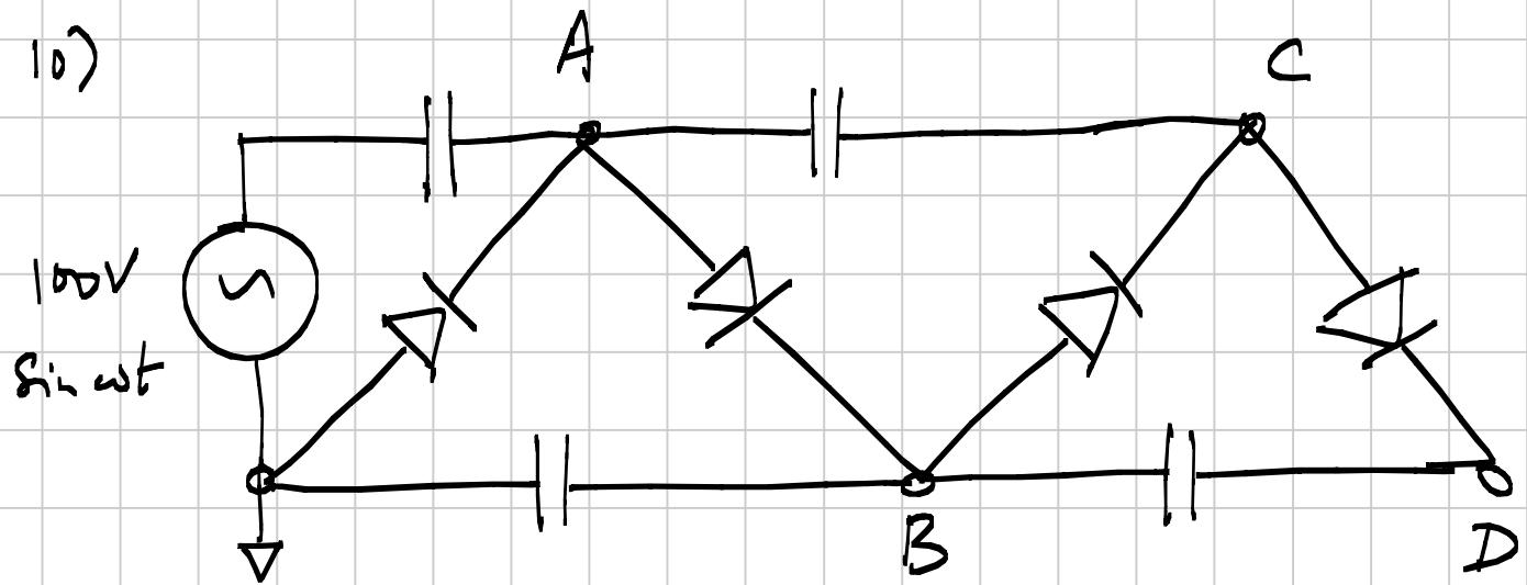
$\omega = 2\pi 50 \text{ Hz}$ . The diodes are ideal.
