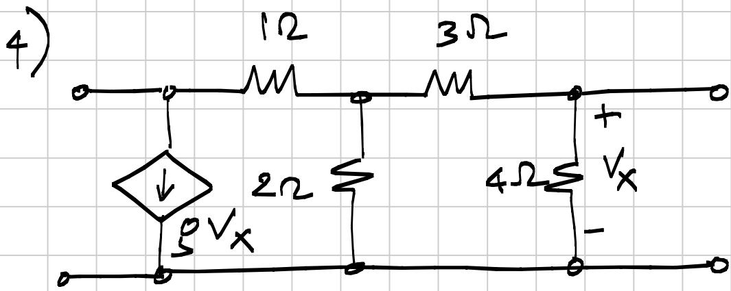
What do you understand by a unilateral two port? What constraint(s) does it impose on the y-matrix? The network above needs to be made unilateral. Determine "g" for this to happen.
