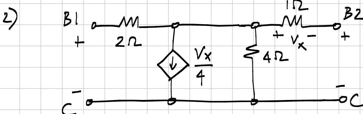
Determine the  $y$ -parameters of the network above.
