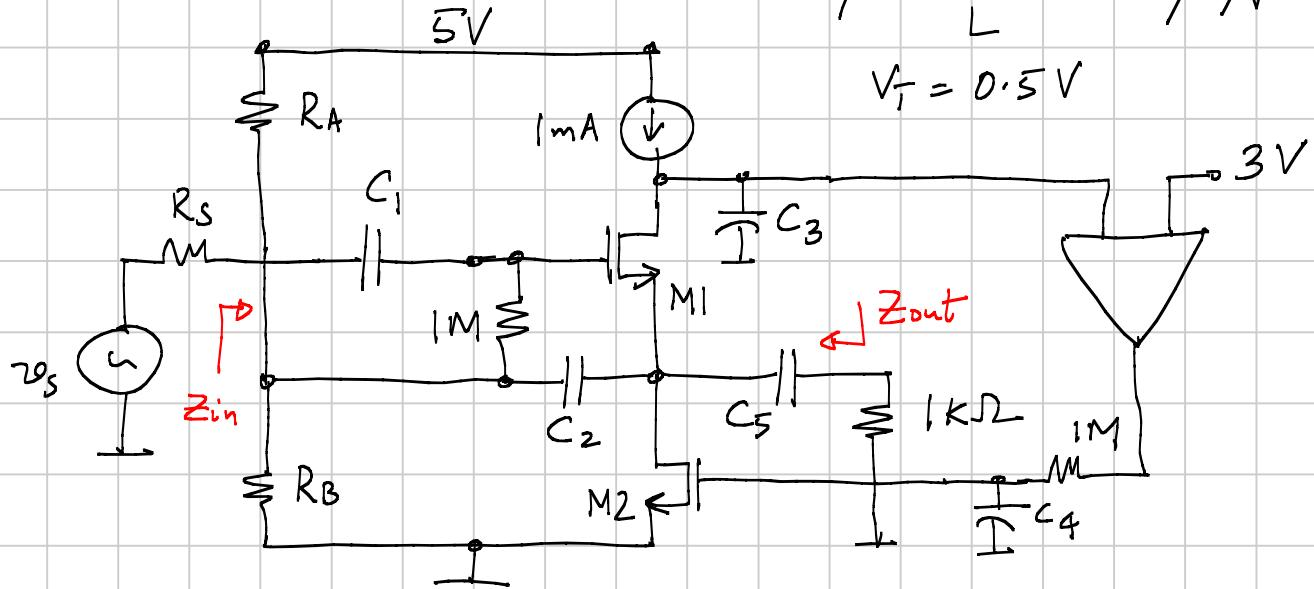
The circuit above shows yet another way of stabilizing the operating point of a transistor. The opamp is ideal.
