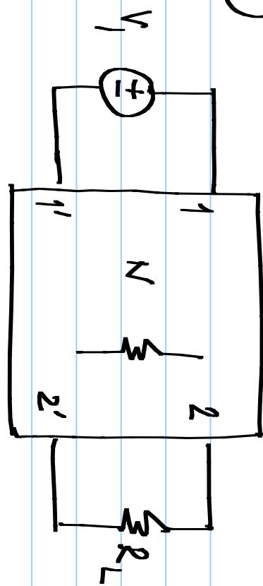
$N$  consists only of resistors. The power in  $R_L$  equals 8W
