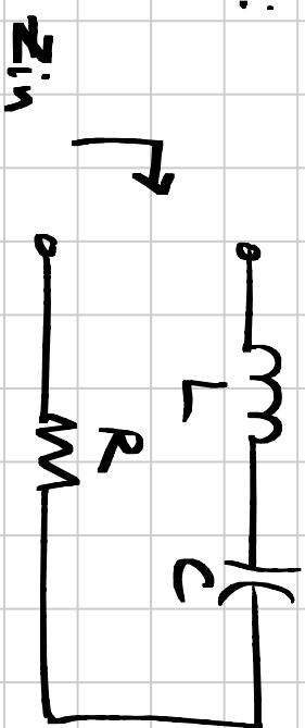
The series RLC network is excited by a voltage at the resonant frequency.
