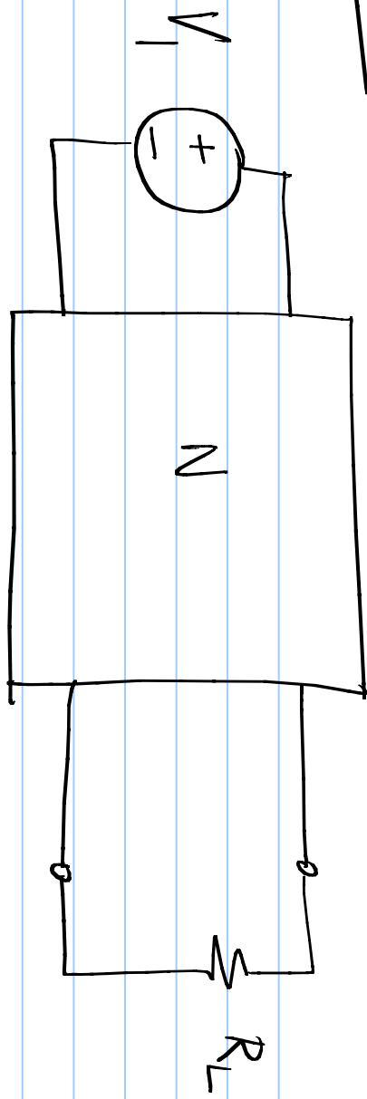
$N$  is a network with resistors only. It is observed that the power dissipated in  $R_L$  is equal to 8W when  $R_L$  is either  $25\Omega$  or  $100\Omega$ . Determine the power dissipated in  $R_L$  when  $R_L = 75\Omega$ .
