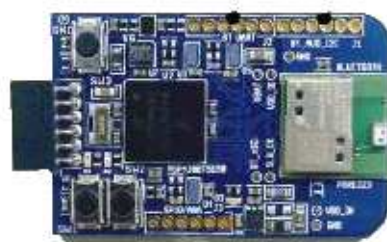
Figure 3.5: Bluetooth transceiver EZ430RF2560 [12].
