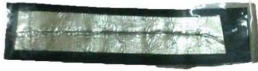
Figure 4.4: The velostat layer is sandwiched between two layers of aluminium foil. Contact wires are yet to be placed.
