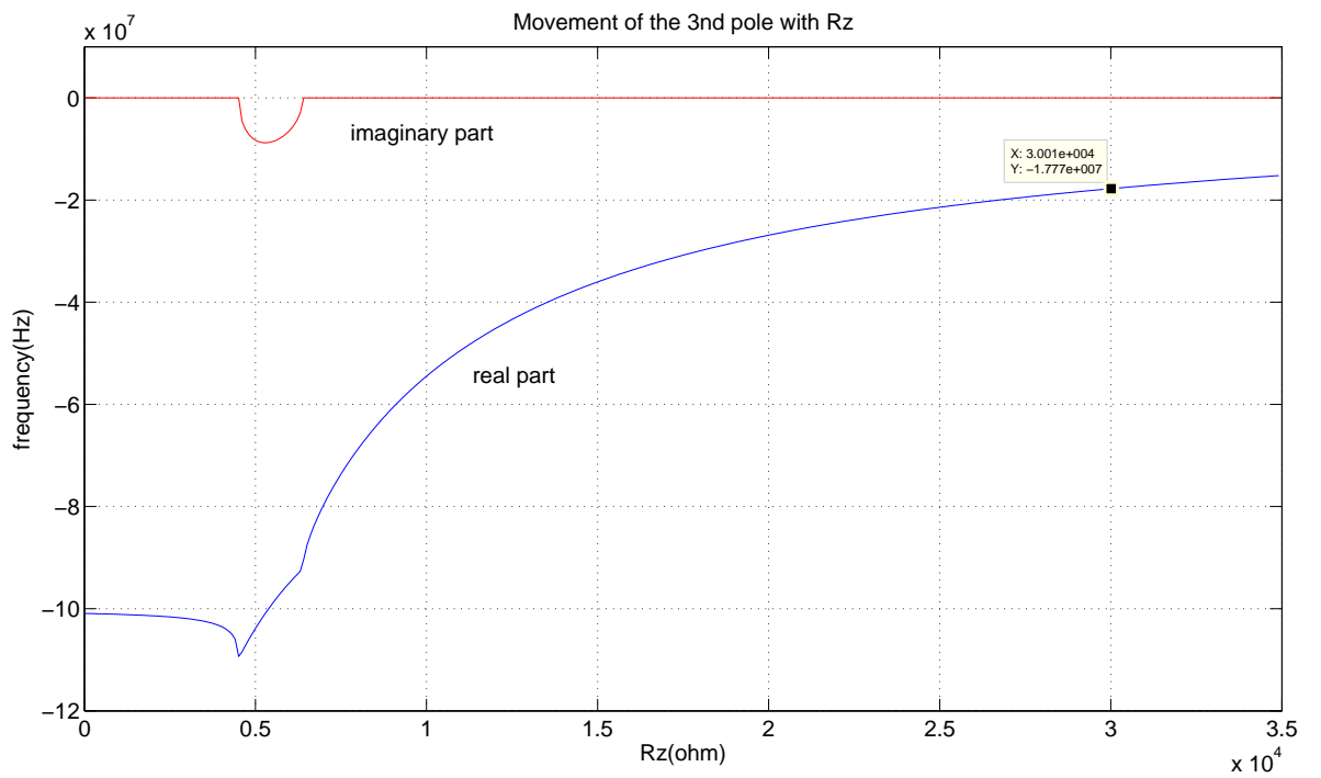
Figure 4.9: Movement of the 3rd pole with variation of R_z .
