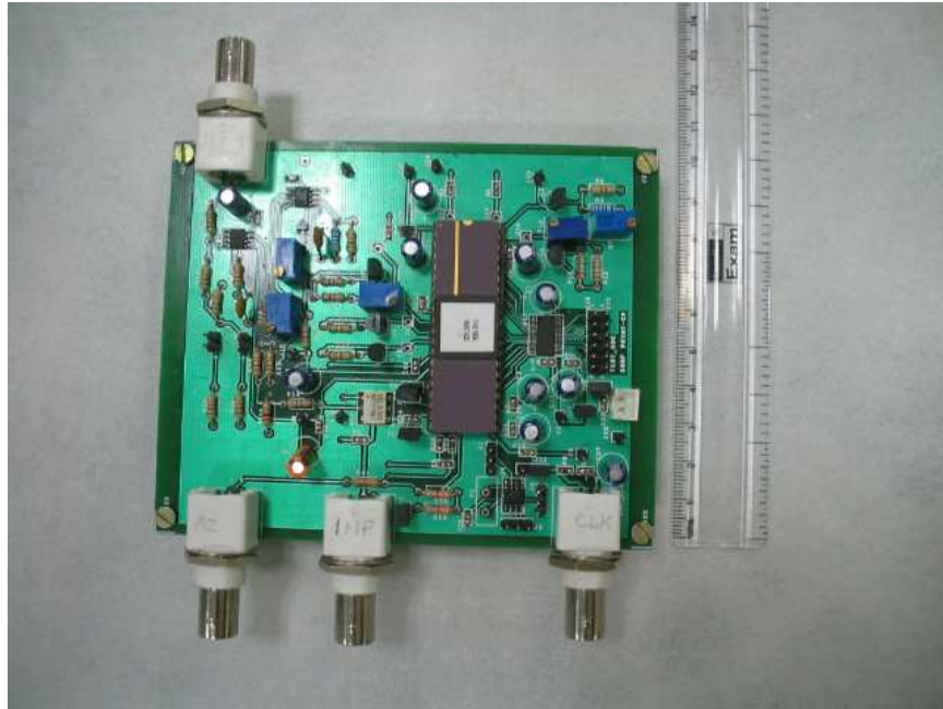
Figure 12.1: The PCB designed for testing the ADC.
