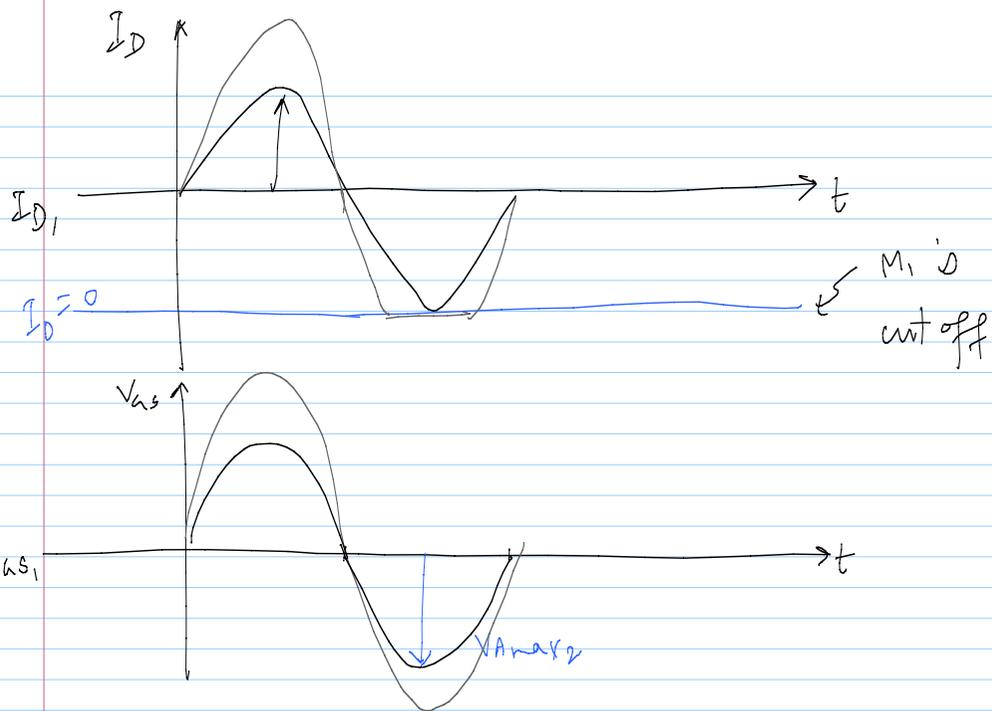
$$I_D = 0 \text{ when } |I_{D,1}| = |g_m V_{A_{max,2}}|$$
