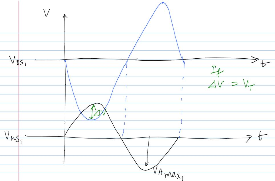
$V_{A_{max,1}} \equiv$  Maximum value of  $V_A$  that keeps  $M_1$  from going into triode region at any time (positive half cycle)
