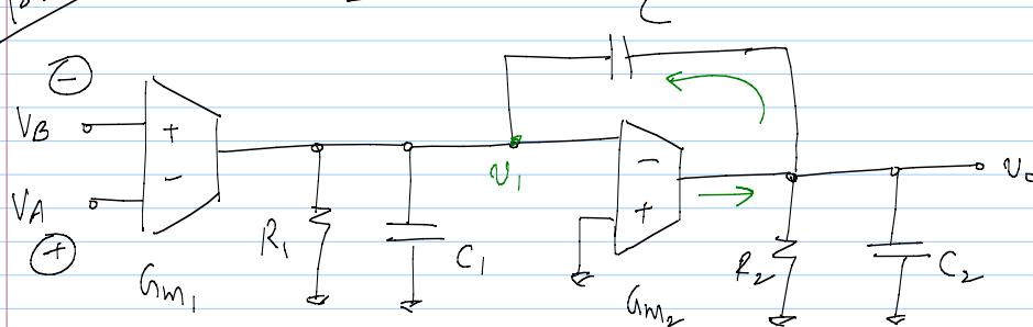
$$\frac{V_o}{V_{i-A}}(s) = -G_{m1} G_{m2} R_1 R_2 \left[ \frac{sC}{G_{m2}} - 1 \right] \\ \frac{s^2 [CC_1 + C_1 C_2 + CC_2] R_1 R_2 + s [C \{R_1(1 + G_{m2} R_2) + R_2\} + R_1 C_1 + R_2 C_2]}{+ 1}$$
