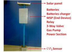
Figure 3: A CO<sub>2</sub> sensing WSN node.
