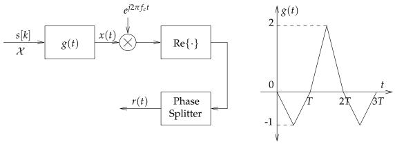
Assume a symbol rate of  $\frac{1}{T}$  and carrier frequency  $f_c = \frac{3}{T}$ . Let  $\mathcal{X} = \{1, -1, j, -j\}$  and consider the transmission of the three-symbol sequence  $s[k] = \{1, -j, j\}$ . The phase splitter nulls all negative frequencies in the signal. (continued in next page)
